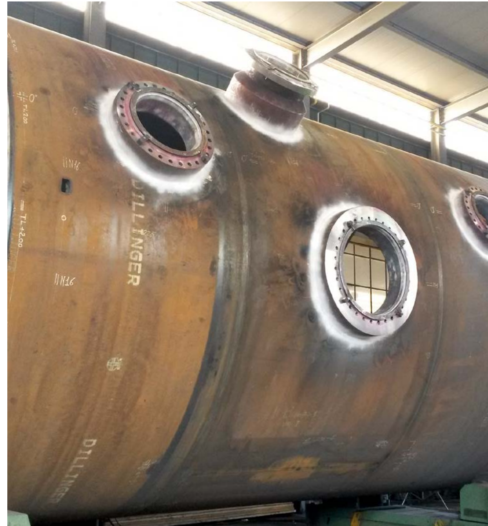
Çöpler autoclave shell in fabrication
