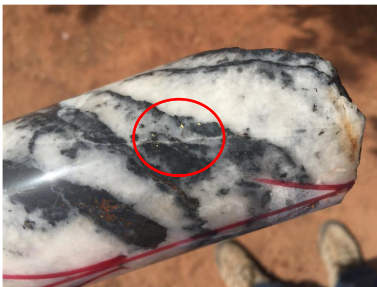
Figure 5: Drill core from DDDK16-002. Later stage quartz vein with visible gold (circled) and fragments of footwall graphitic sediments
