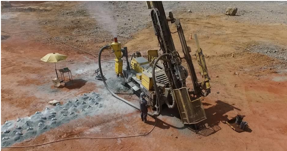
Grade Control Drilling –Stage 2 pit
