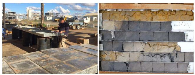
Figure 1: Logging and Sampling of Sonic Core - Holes HMI063S and HEX019S shown
