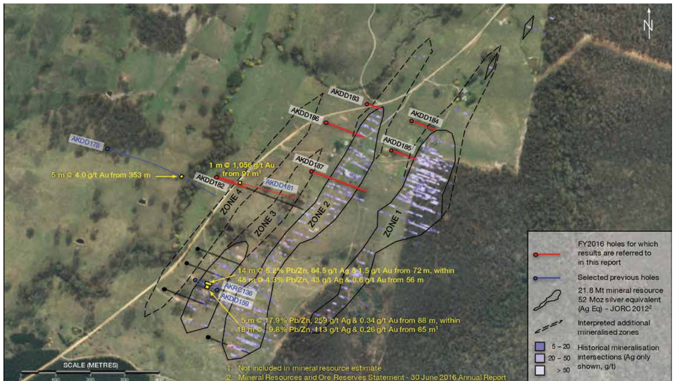
Figure 5 – Plan view of selected hole and intersection locations
