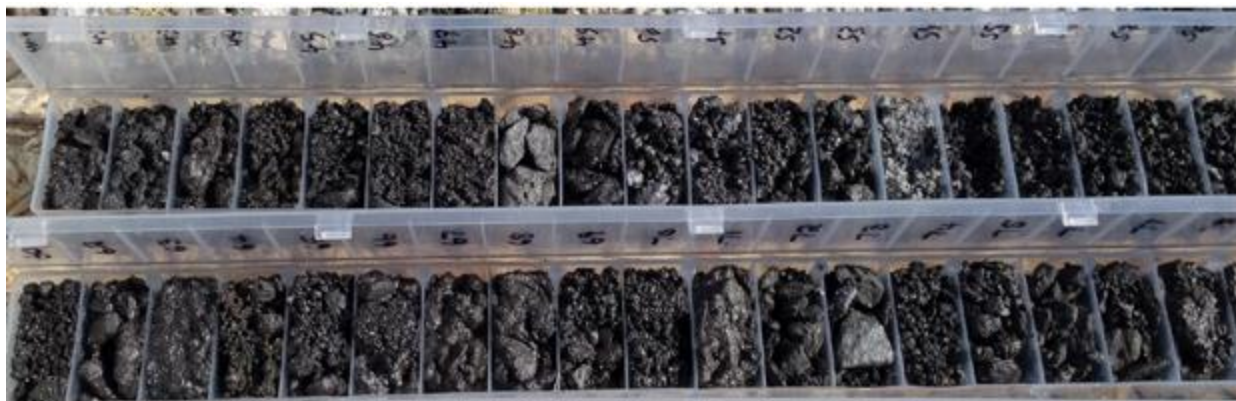
Figure 2. One metre drill samples of graphite mineralisation from hole SIV056 (from 40 to 80m)
