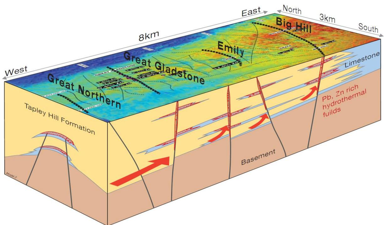
Figure 1. Conceptual block model with magnetic image showing mineralised structures that have been mapped, sampled and drilled, and potential large-scale stratiform zinc targets, Yerelina, SA.
