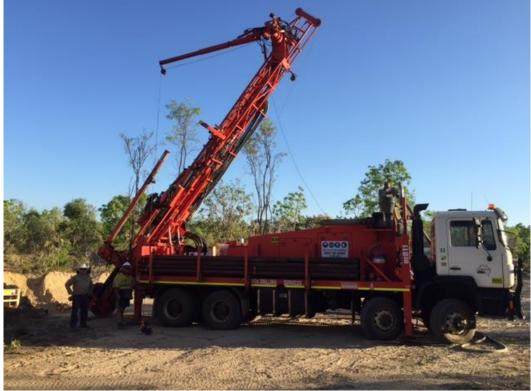
Figure 1. RC Drill rig at BP33, Finniss Project, NT
