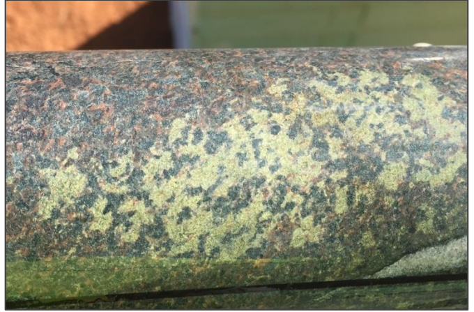
Photo 3: 159m - epidote replacement of feldspars (Scale: core diameter 61mm)
