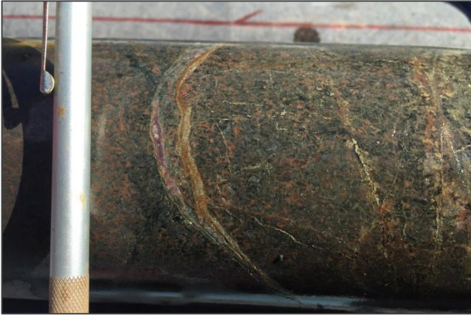
Photo 2: 54m downhole - rhodocrosite vein & pyrite network veins in haematite altered monzonite porphyry (Scale: core diameter 61mm)
