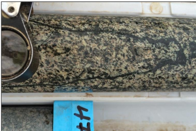
Photo 6: 474m - magnetite veinlet in sericite biotite altered monzonite (Scale: core diameter 51mm)
