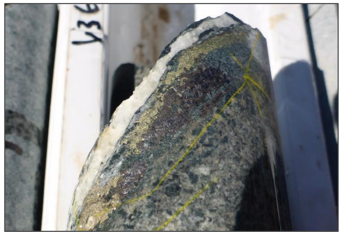
Photo 5: 360m - carbonate pyrite chalcopyrite sphalerite vein in altered monzonite with chlorite altered feldspars (Scale: core diameter 51mm)
