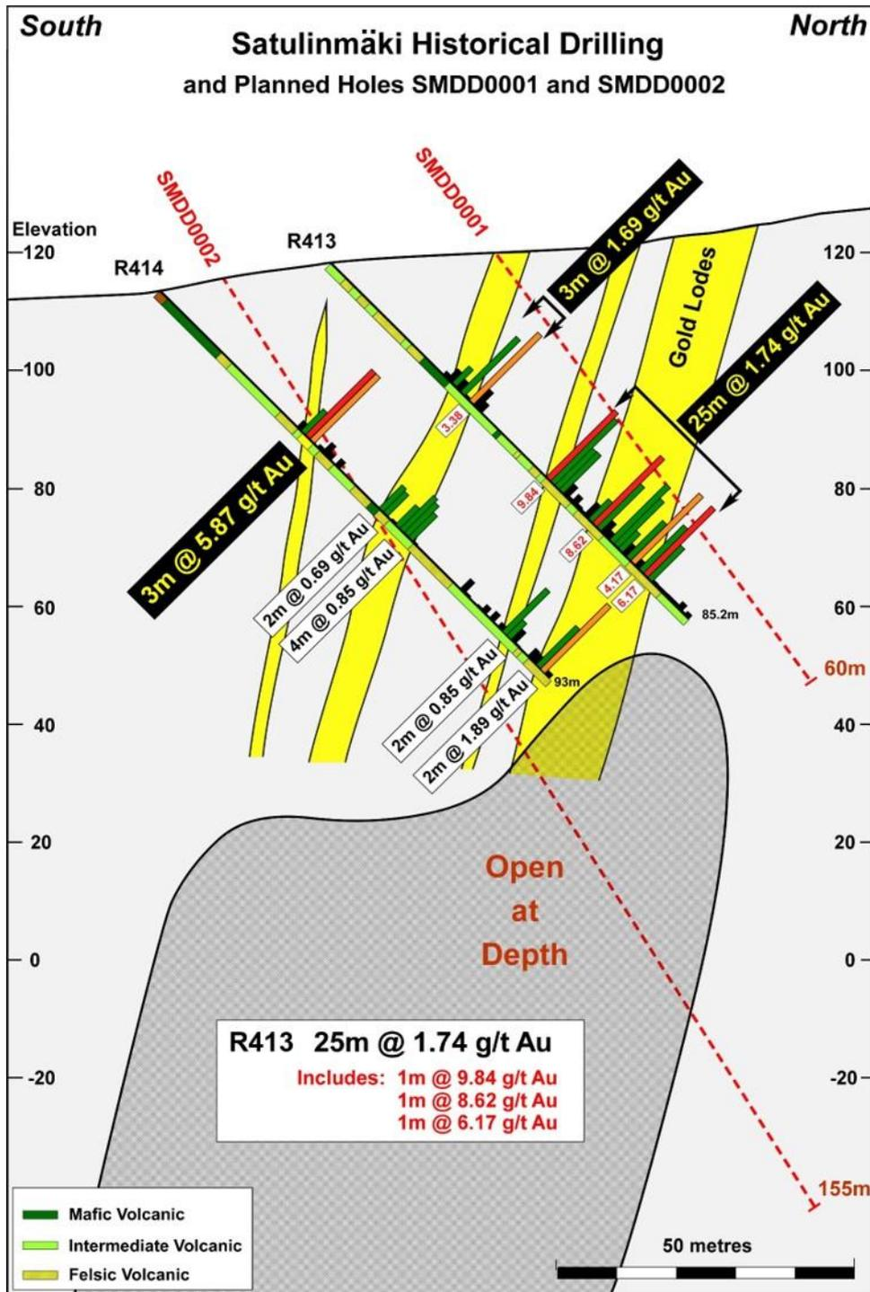
Figure 3: Cross section showing target zone down plunge from mineralised horizons in historical holes R413 and R414.
