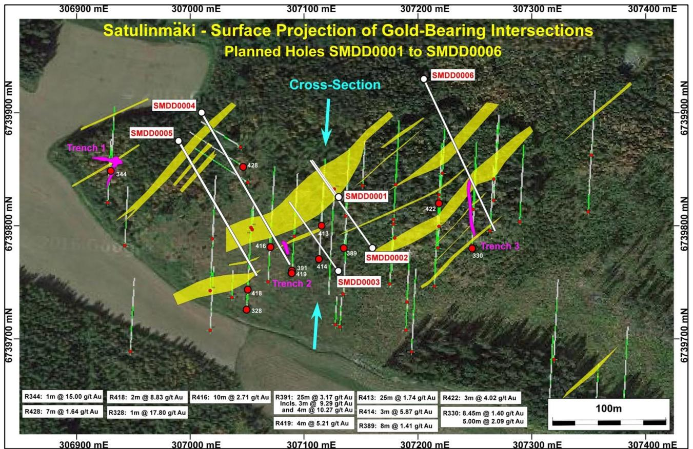
Figure 2: Satulinmäki gold prospect showing interpreted NE trending gold bearing vein systems. Figure 3 cross section is shown through the main target vein. Collar positions of historical holes with red dots and grey, green traces. Proposed holes SMD001 to SMD006 are shown in white.
