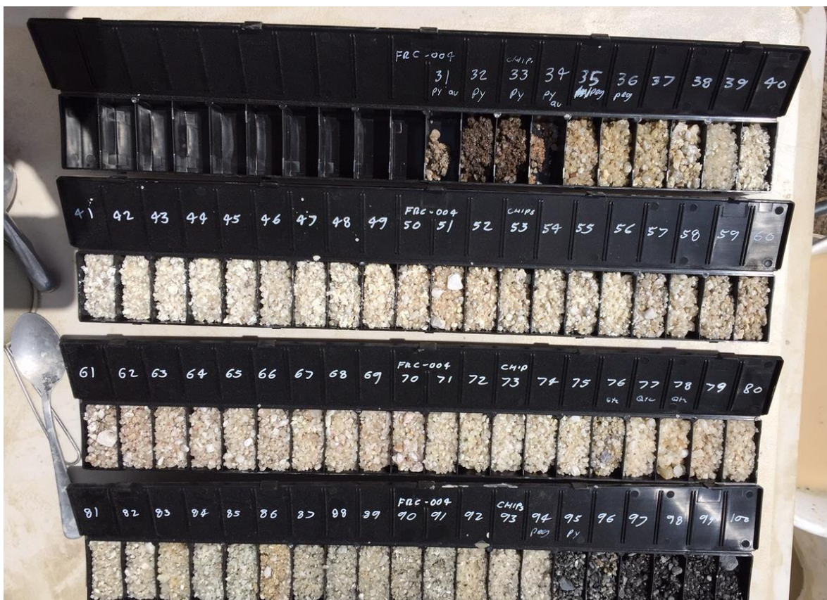
Figure 1. Sieved RC drill chips of pegmatite intersection (34m-94m) drillhole BPRC004 BP33 Pegmatite, EL 29698, Finniss Lithium Project, NT.
