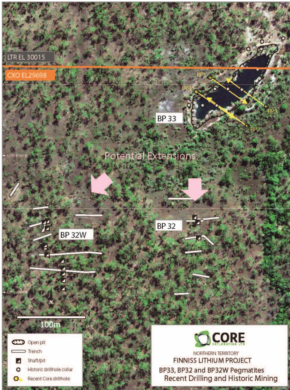
Figure 3. BP33, BP32 and BP32W Pegmatite locations showing recent drilling and previous mining, drilling and trenching work, Finniss Lithium Project, NT.
