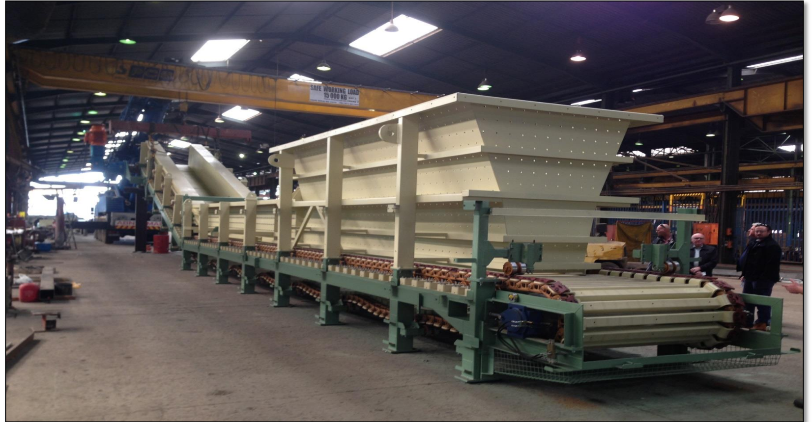
Above: Low profile loader to replace CV06 to transfer crushed material from crusher to crushed ore stockpile
