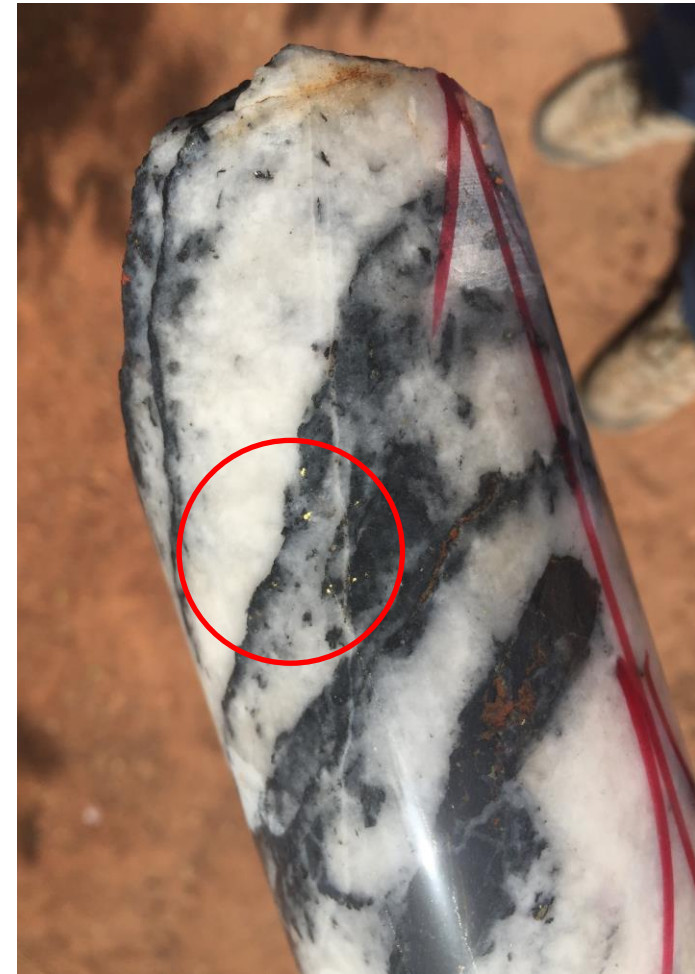
Drill core from DDDK-16-002, later stage qtz vein with visible gold
