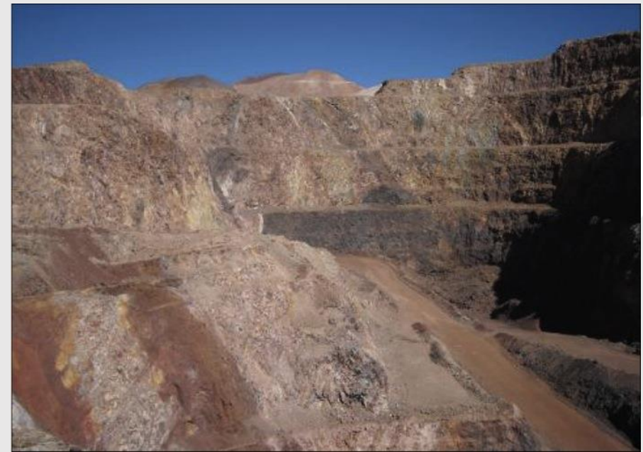
West wall of Chimberos pit showing oxides assoc. with mineralisation
