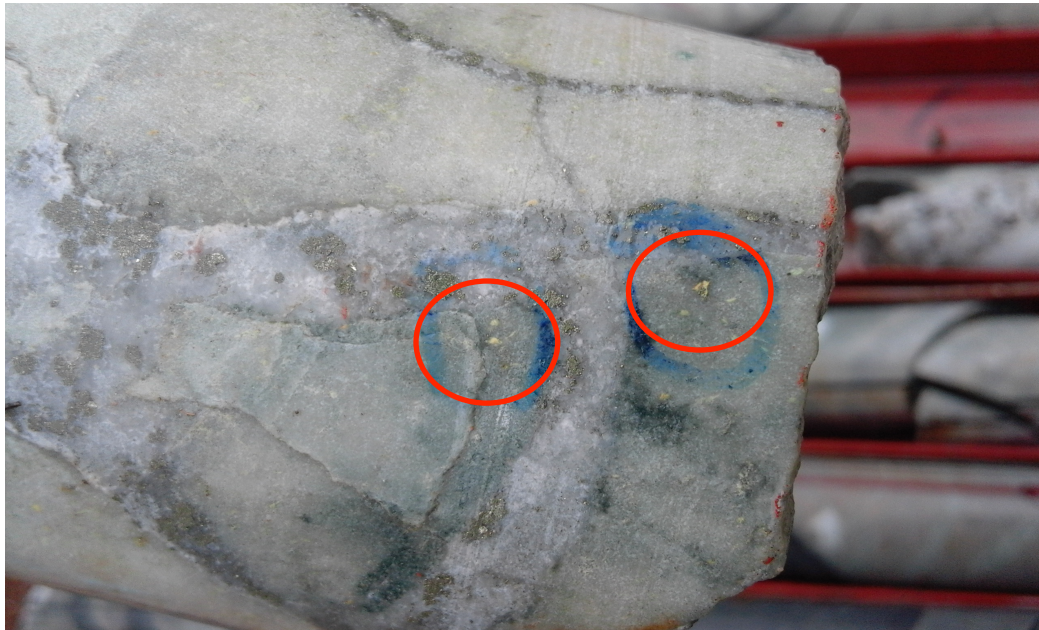
Figure 4: Drill core from DDDK16-004 showing visible gold (circled) at 164.9m depth.
