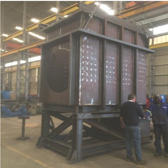
Left: Newly designed SAG Feed chute
