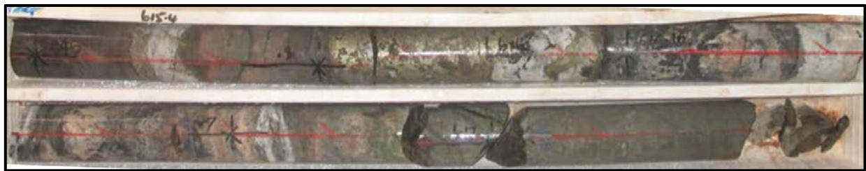
Figure 5: MHC20001 drilled in 2012 (615.80 to 616.16m) Minyari brecciated chalcopyrite-quartz-calcite vein similar to the Telfer mineralisation assemblages (0.36m at 41.55 g/t gold, 12.02% copper and 43.80 g/t silver).
