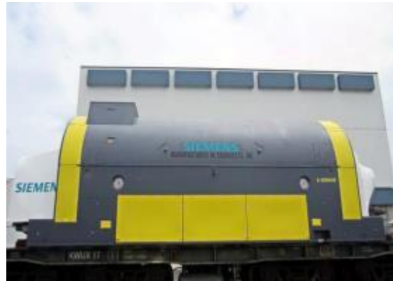
Steam Turbine Generator
