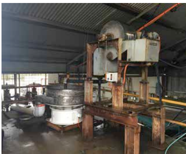
Figures 1A & 1B: Commissioning the magnetic separator and sizing screen & flotation cells
