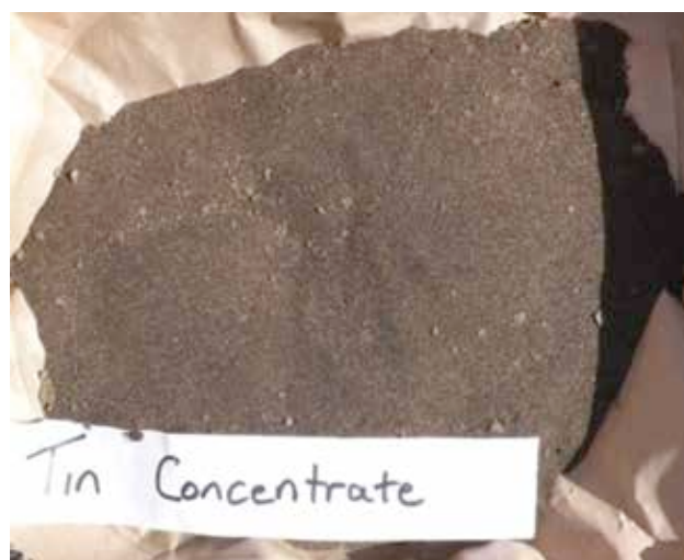
Figures 1C & 1D: Commissioning the dressing table and final 55%Sn concentrate (dried)
