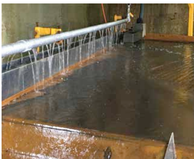
Figures 1C & 1D: Commissioning the dressing table and final 55%Sn concentrate (dried)
