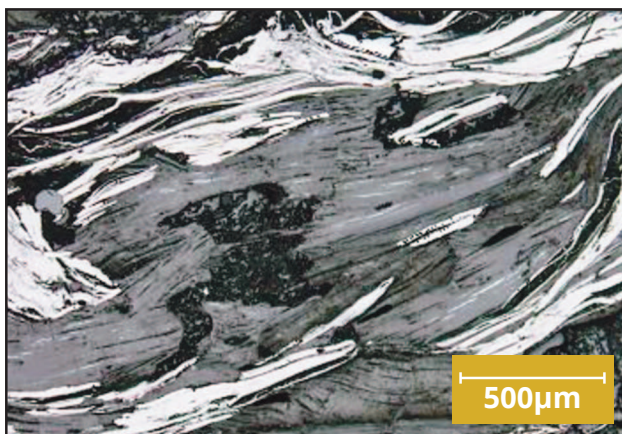
Figure 7. Photomicrograph of graphite flakes (in white) from Siv014 (17m to 18m)
