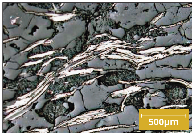
Figure 8. Photomicrograph of graphite flakes (in white) from Siv002 (92m to 93m)
