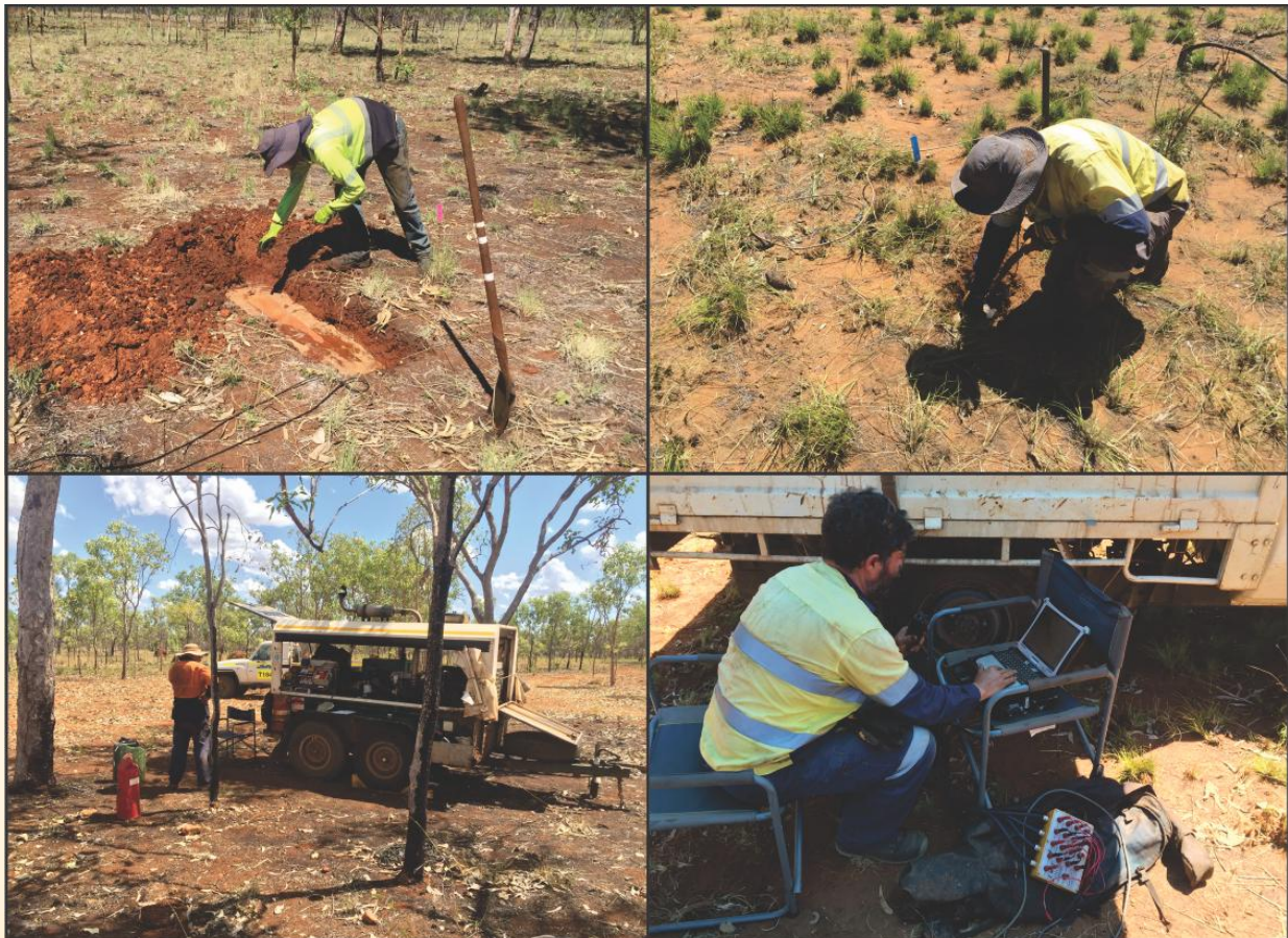
Figure 6 – Photographs of field personnel from Moombarriga Geoscience undertaking the Pseudo 3D Induced Polarisation and Resistivity survey at Merlin Prospect, Double Magic Project, September 2015. The two left side images depict transmitter setup, those on the right side, receiver setup.
