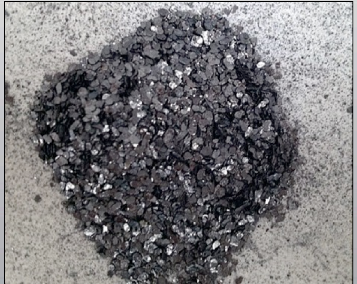
Extra large coarse flakes ( \gg 600\mu\text{m} ) from diamond core hole (CRD090) at Siviour prospect
