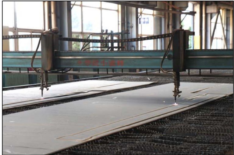
Laser cutting of steel, subcontractor factory Dalian
