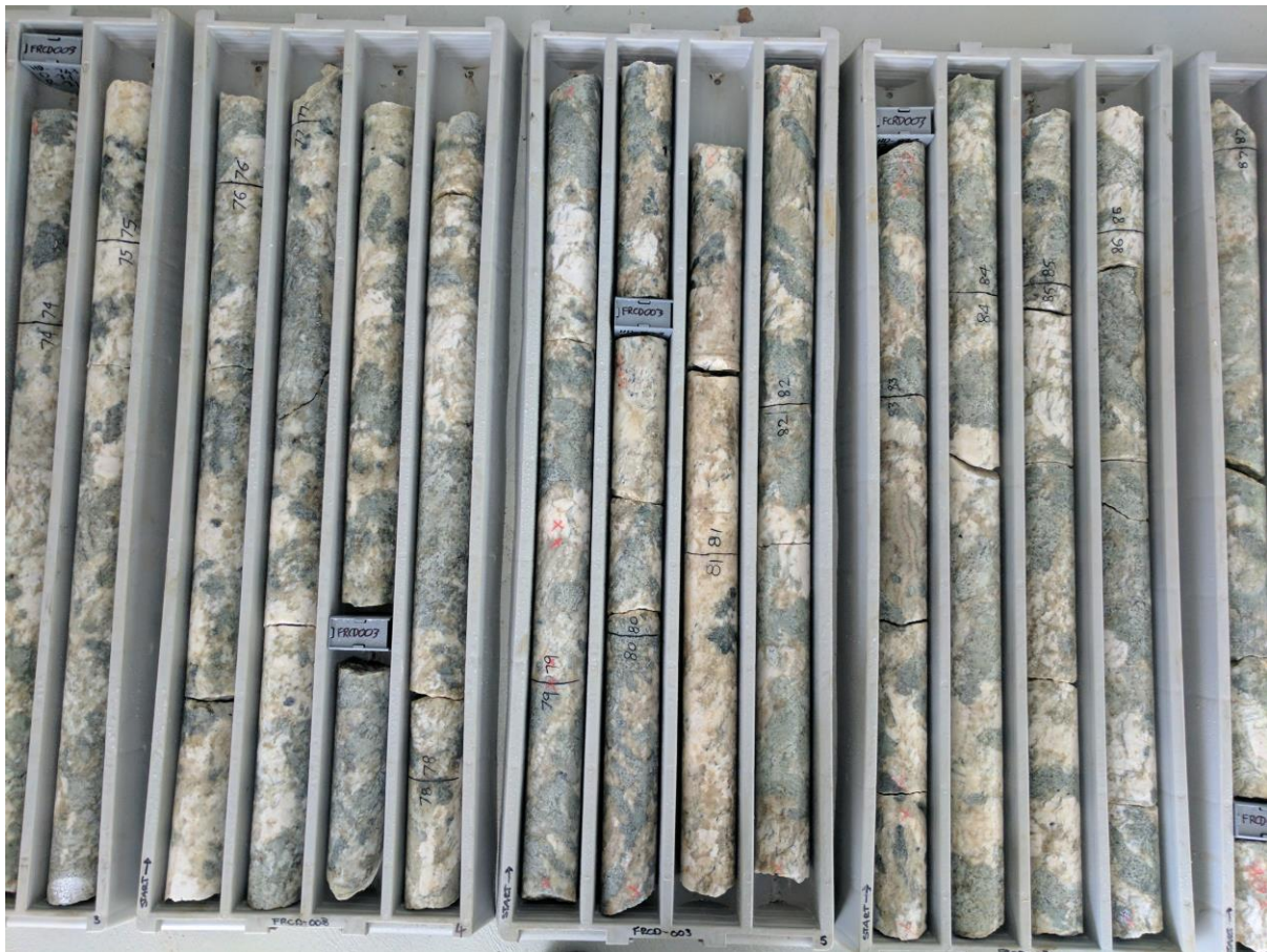
Figure 3. Large green spodumene crystals making up a high proportion of pegmatite volume hosted by lighter coloured (white) feldspar and quartz 73.8m – 87.1m FRDD003 (HQ) Grants Prospect, Finniss Lithium Project, NT.
