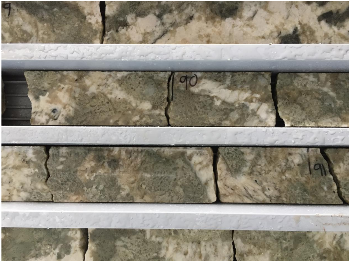
Figure 2. Large green spodumene crystals making up a high proportion of pegmatite volume hosted by lighter coloured (white) feldspar and quartz. 89m – 92m FRDD002 (HQ), Grants Prospect, Finnis Lithium Project NT.
