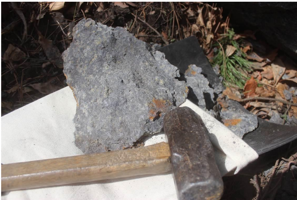
Figure 2: High-grade flake-graphite sample from outcropping graphitic unit at Yongwon (16% TGC D1 )
