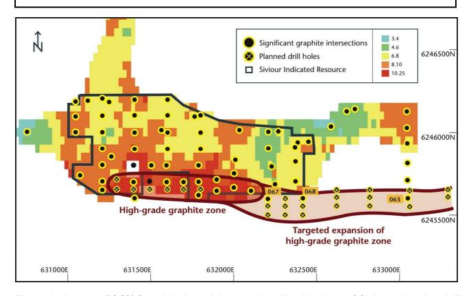
Figure 1. Average TGC% from block model over mineralised horizon of Siviour, showing drill holes within block model and targeted expansion zone and planned drill holes
