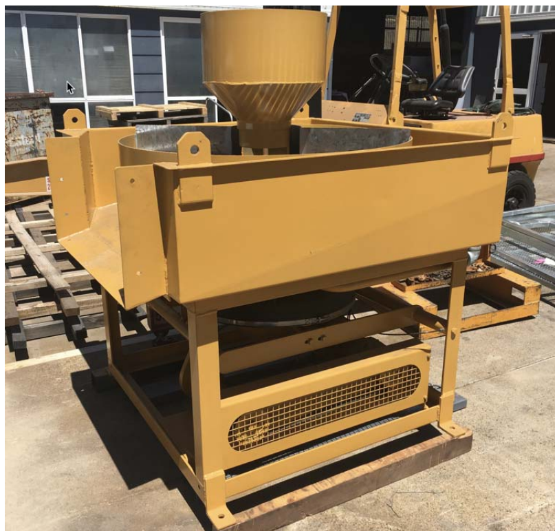
Figure 1 – Primary jig for first stage concentration of tin
