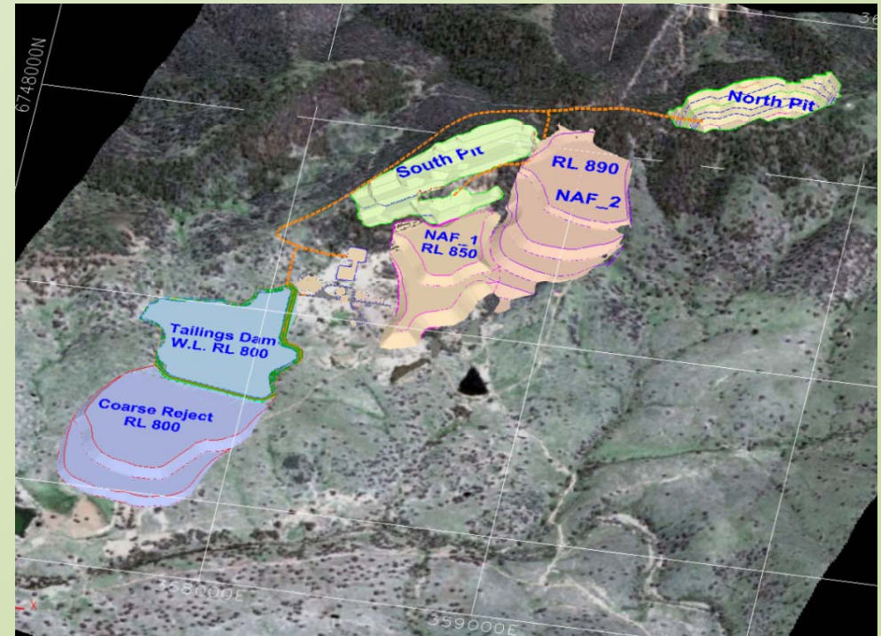
Schematic of Taronga life of mine pit shells and associated infrastructure
