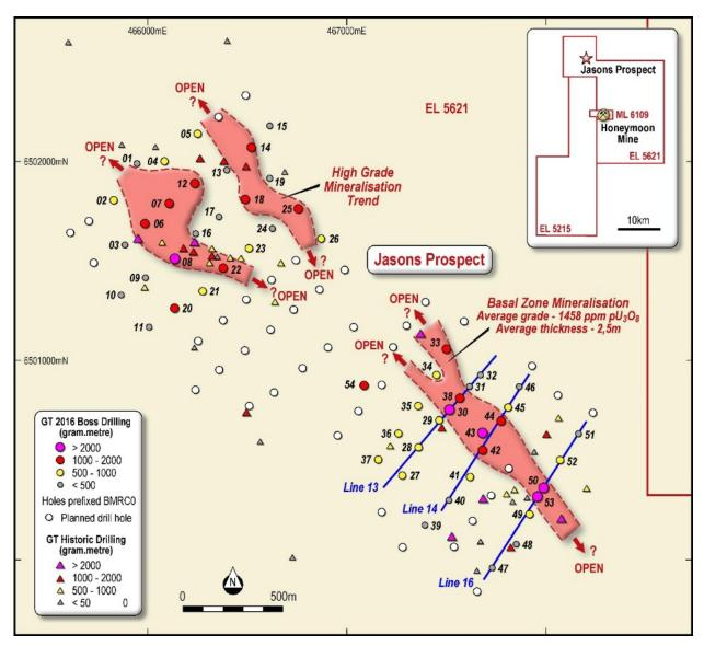
**Figure 1:** Location of drilling at the Jasons Prospect, approximately 15km north of the Honeymoon Mine site. Maximum grade times thickness (eU3O8 [in ppm] x m) shown to assist in illustrating high-grade trends.
