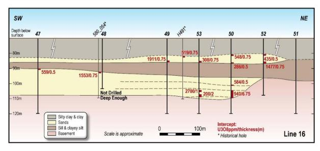
Figure 2: Example cross sections through Lines 13, 14 and 16. Results are shown as grade (ppm  $eU_3O_8$  or  $pU_3O_8$  / thickness in metres where available). Note: sections only show the bottom ~60m of each section.
