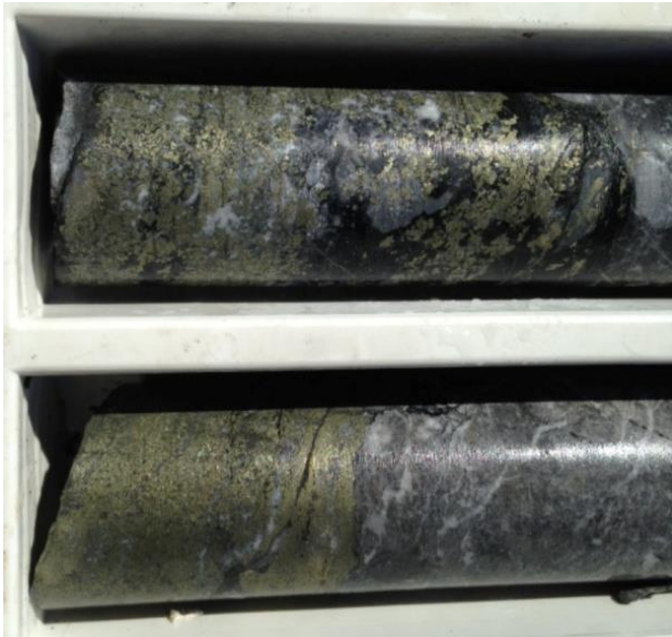
Figure 2: Drill core CCD03 – semi-massive chalcopyrite bands
