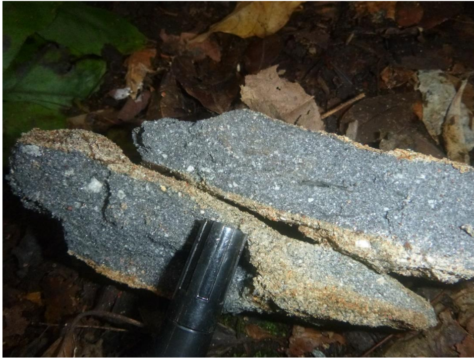
Figure 2: Sample MKR160 from the Dikaki Prospect returned an assay of 29.8% combined Zn+Pb.
