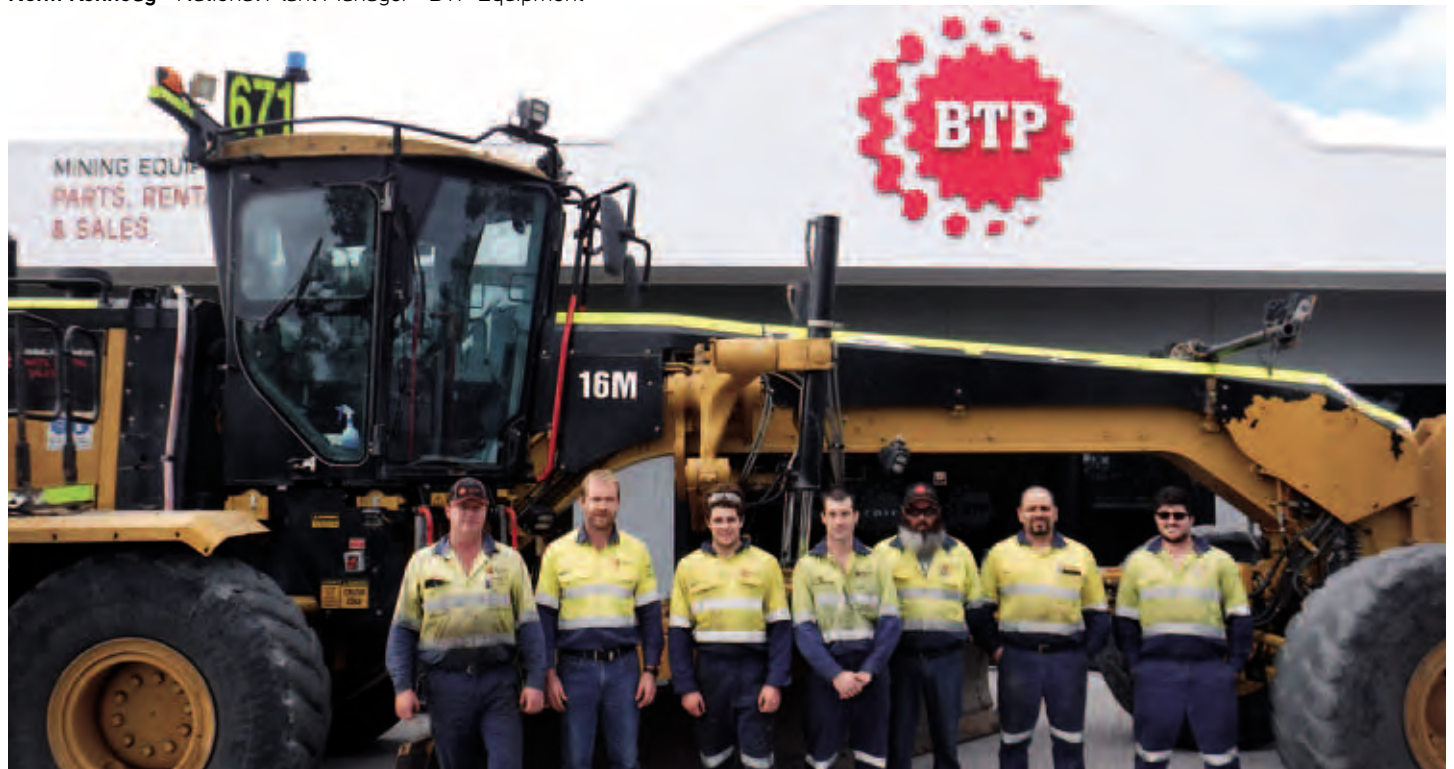
16M Grader going back to Wambo Coal operations after a powertrain rebuild at BTP NSW branch. (L-R Adam Cameron, Dean Garland, Joe Wilton, Jason Hewitt, Shaun Murphy, Joe Farrugia, Matthew McCullough)
