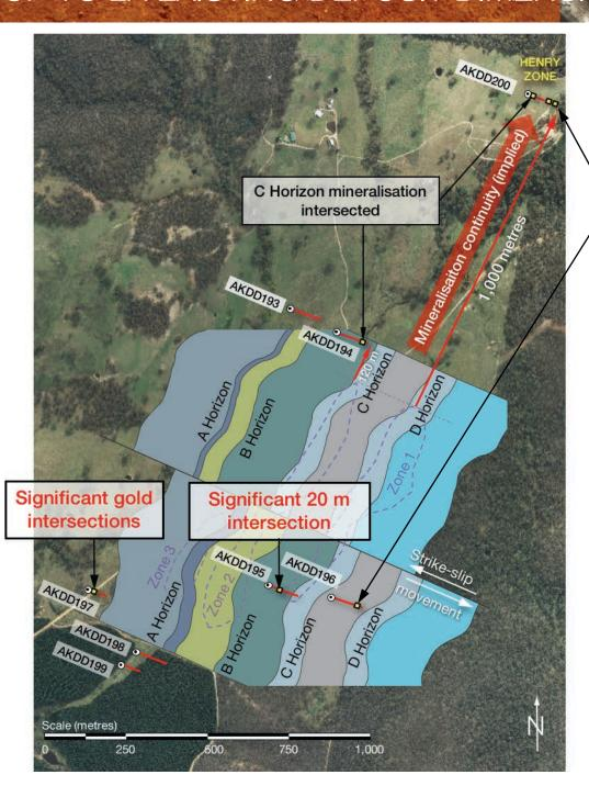
The Kempfield geological model confirmed by 2016/17 diamond drilling.
