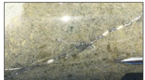
12. PPDH155/143m: Carbonate vein with lead and zinc sulphides cutting altered monzodiorite.
