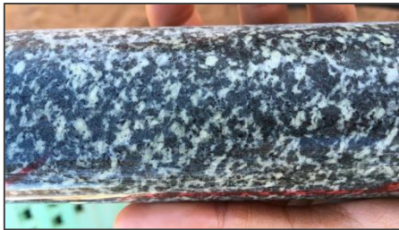
4. PPDH155/404m: Biotite alteration with disseminated fine chalcopyrite (not visible).
