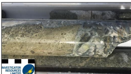
13. PPDH155/247m Brecciated chalcidony veins cutting intense sericite alteration.
