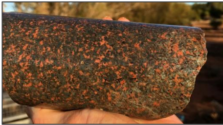
1. PPDH157/55m: Potash feldspar biotite magnetite haematite altered monzodiorite.
