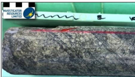
10. PPDH155/104m: Fine repetitive hairline fractures in sericite-altered monzodiorite.
