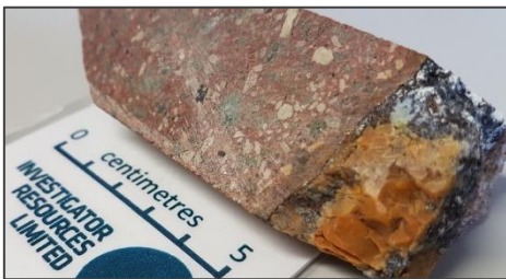
7. PPDH156/55.2m: Kaolinite (possibly after pyrophyllite) gossan (oxidised sulphides) vein in altered monzodiorite.
