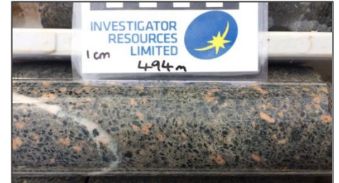
6. PPDH157/494m: Scattered potash feldspar alteration & quartz veining. Disseminated sulphides are <1%.
