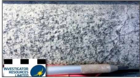
8. PPDH155/40m: Kaolinite illite topaz fluorite pyrite alteration. Some of the dark minerals are silver & copper chlorides (SEM probe).
