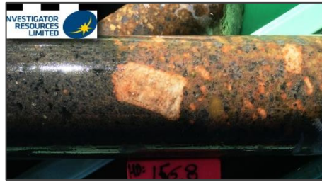
2. PPDH155/157m: Remnant potash feldspar biotite alteration.
