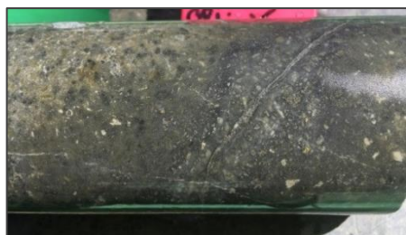
11. PPDH155/132m: Altered monzodiorite with feldspar outlines preserved in sericite ground-mass, cut by multiple zoned pyrite veins.
