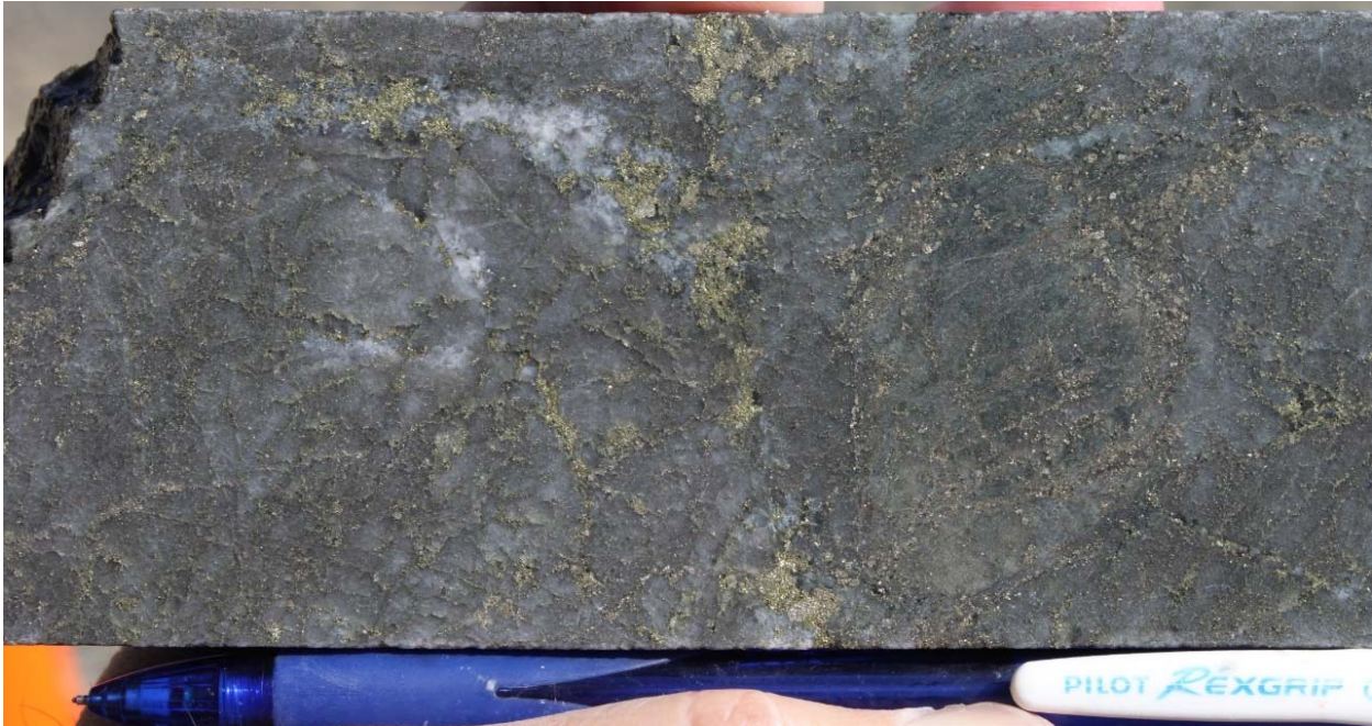
Figure 14: Core photo at 347m down-hole showing the mineralisation style intersected in TMMRD006
