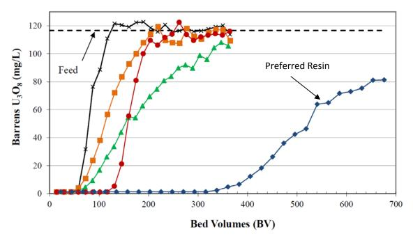
*Figure 1: Uranium Breakthrough Curves* (4.0-4.6 BV/hr, 30 deg C, pH 1.8, 8,8g/l Cl)
