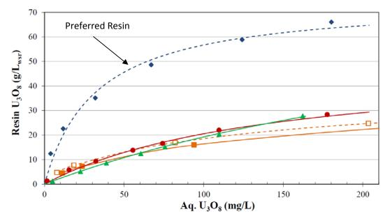
Figure 2: Uranium Loading Curves (30 deg C, pH 1.7-1.8, 8,8g/l Cl)
