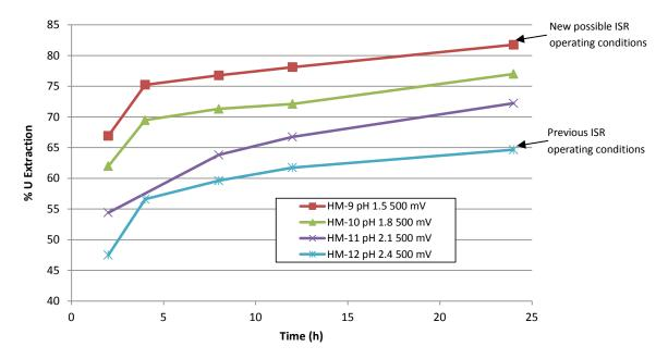
Figure 3: Effect of pH on Uranium Extraction from High Clay Sample
