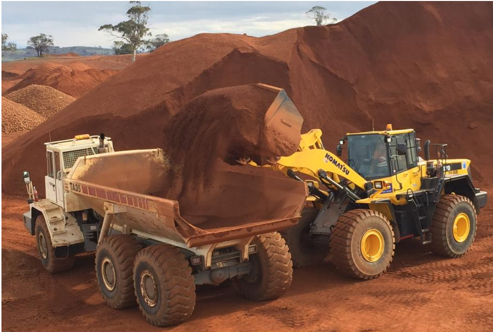
Figure 6 Blending cement-grade bauxite at Bald Hill Mine Site
