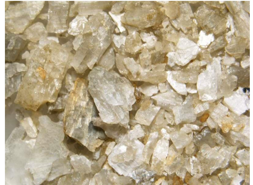
8.1% Li 2 O Spodumene Concentrate from HLS Testwork
