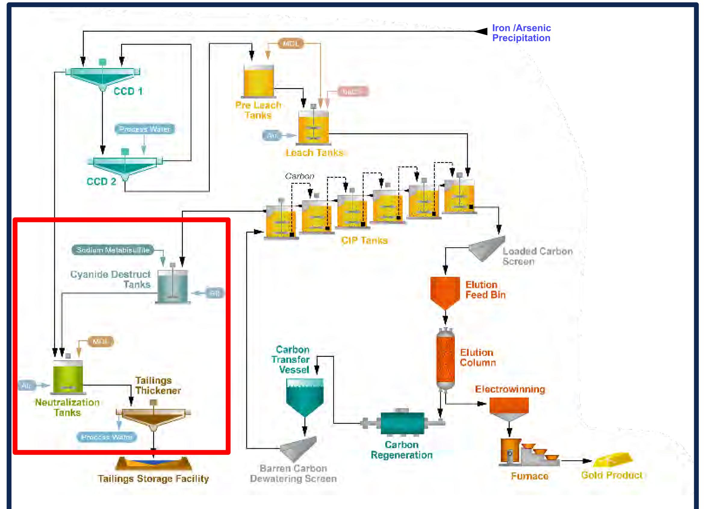
The tailings is thickened and process water is recovered for re-use in the plant, and the fina detoxified neutralized and thickened tailings is pumped 4.3 km to the Tailings Storage Facility.
