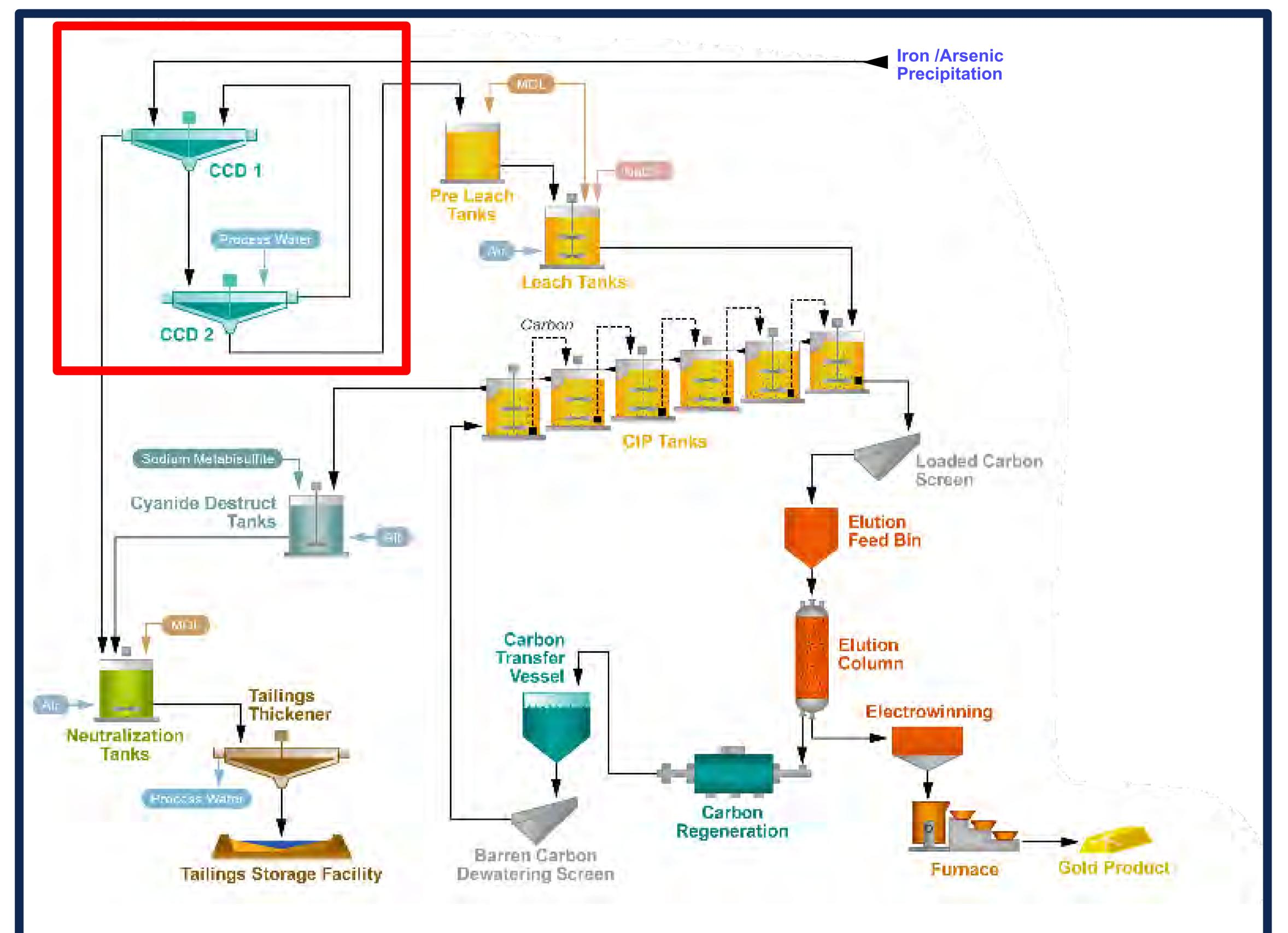
Removing these minerals before the ore is fed into the Cyanide Leach circuit limits cyanide consumption rates.
