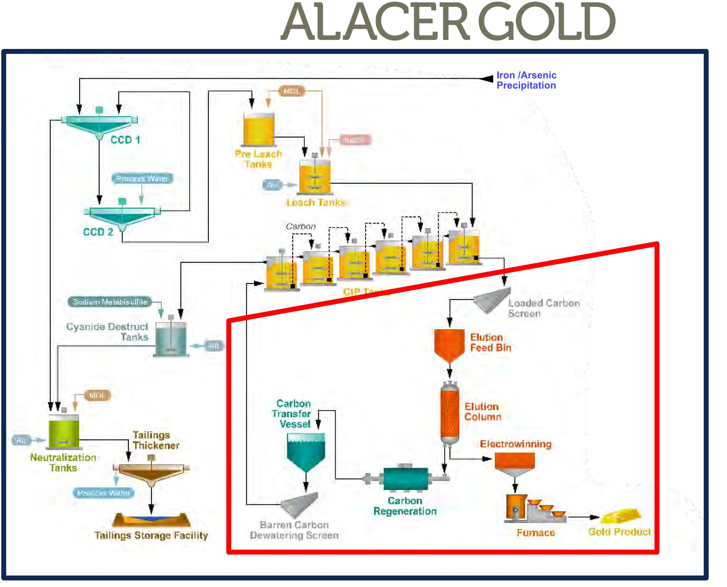
Barren carbon is regenerated in an oil-fire rotary kiln before being returned to the CIP circuit.
