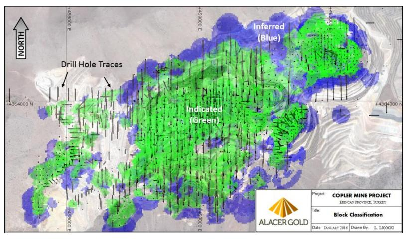
Plan of Resource Classification showing Indicated (Green) with Inferred (Blue) gold mineralization forming a ring around the Indicated mineralization.
