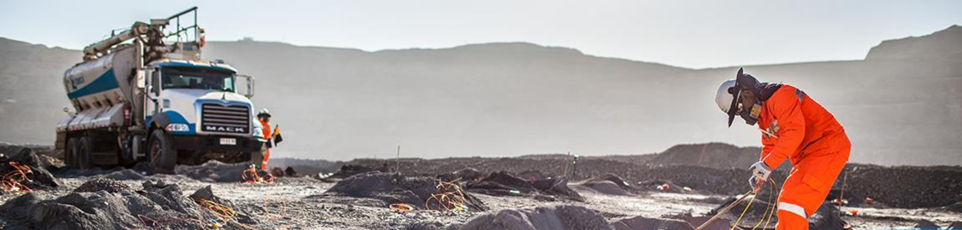
Loading blast holes, Andacollo, Chile
