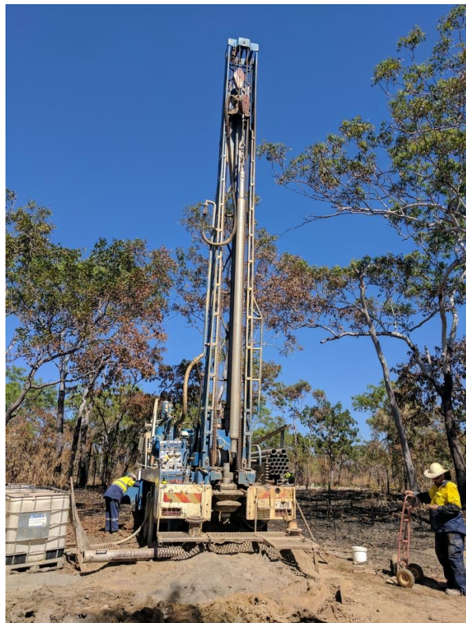
Figure 3. Drill rig establishing groundwater monitoring bores for mine engineering and environmental monitoring purposes, Grants Lithium Resource, NT.
