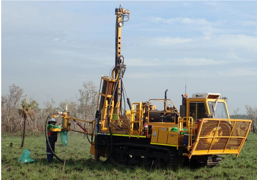
Figure 2. Track-mounted air-core rig drilling shallow exploration holes on “black-soil” plains in the Grants region, Finniss Lithium Project NT.
