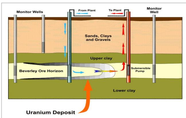
Figure 2: ISR schematic - Beverley mine example.
