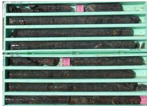
Photo 1: WOMDD001 core 70-77m downhole. Fresh, impermeable metasediment
