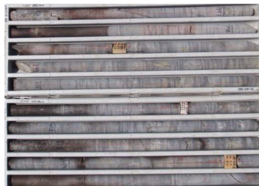
Photo 3: WOMDD001 core 396-405m downhole. Fresh, impermeable metasediment.
