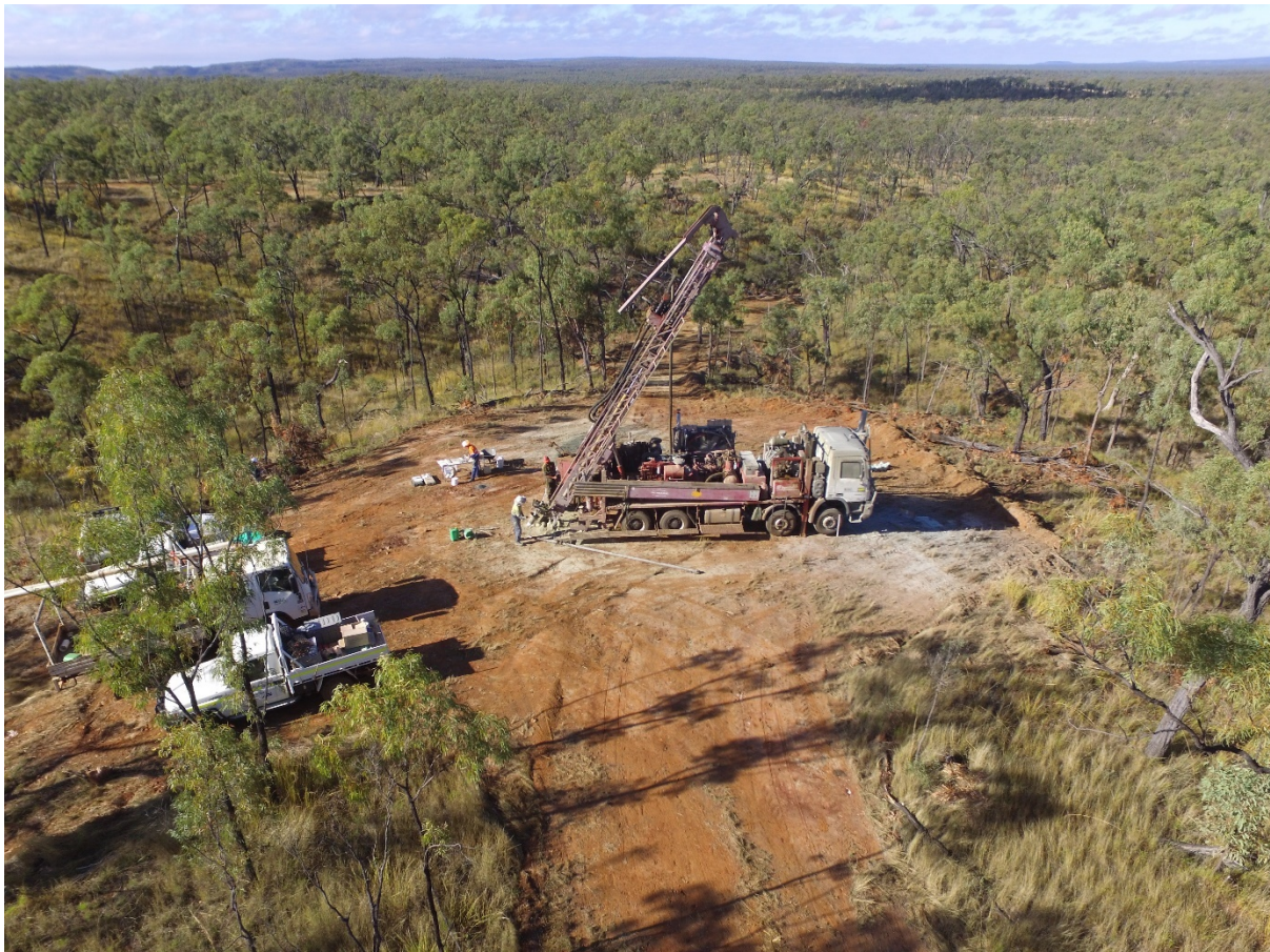
Figure 2. Reverse-circulation drilling at the Company's Bottletree Prospect, July 2017. Aerial view looking southeast.
