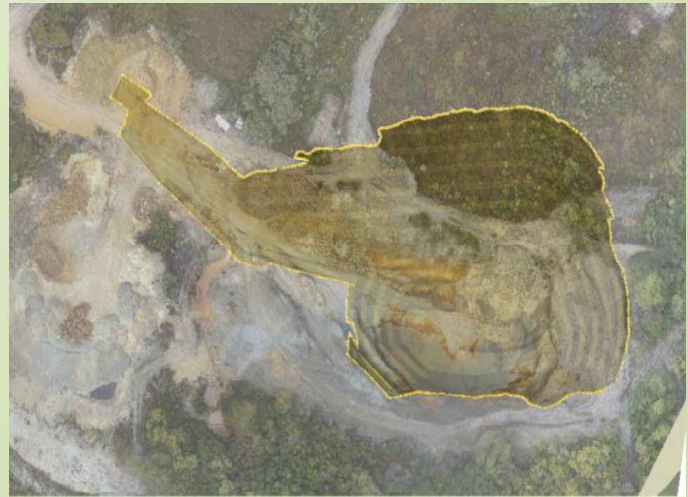
Topographical overview of existing Granville East Mine with proposed east wall cutback superimposed
