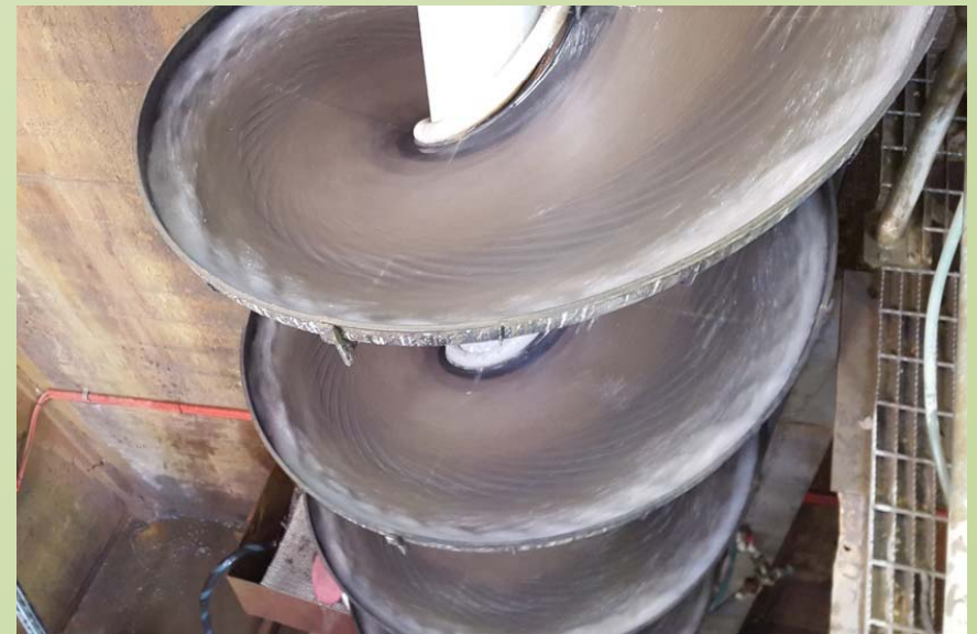
Leading edge Alicoco spiral commissioned July 2017 for fine tin recovery
