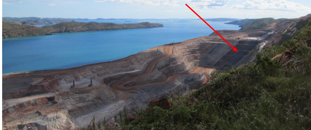
Main Pit in 2014 showing consistency and width of high grade Main Deposit
