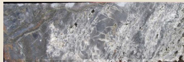
OFDD001: 246m (left) & 248.5m (right) drill core showing strong shearing, qtz veining, pyrite (py) & sphalerite (sp)
