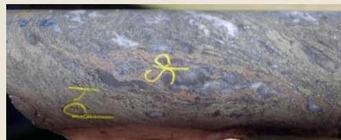
OFDD001: 246m (left) & 248.5m (right) drill core showing strong shearing, qtz veining, pyrite (py) & sphalerite (sp)
