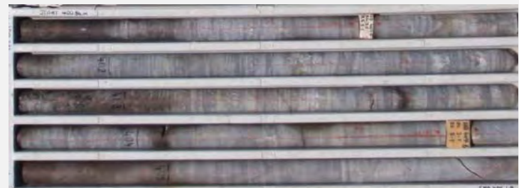
Photo 3 – impermeable fresh rock
