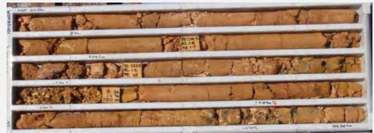
Photo 2 – weathered, porous, permeable? copper mineralised trough material
