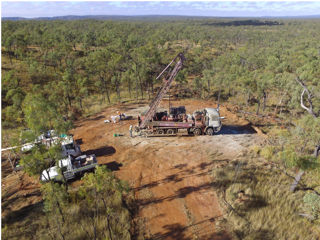
Reverse-circulation drilling (hole SBTRC004) at the Company's Bottletree Prospect, July 2017. Aerial view looking southeast.
