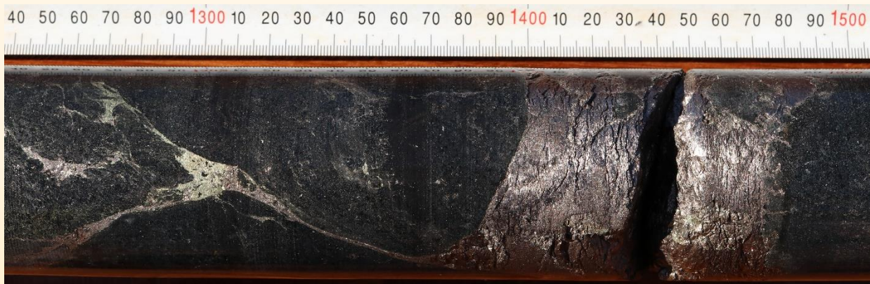
Figure 1 – Stringer and massive sulphide vein in Ruins Dolerite intercepted in DMDD0012, photo is of uncut HQ core, 305.41m to 305.68m downhole
