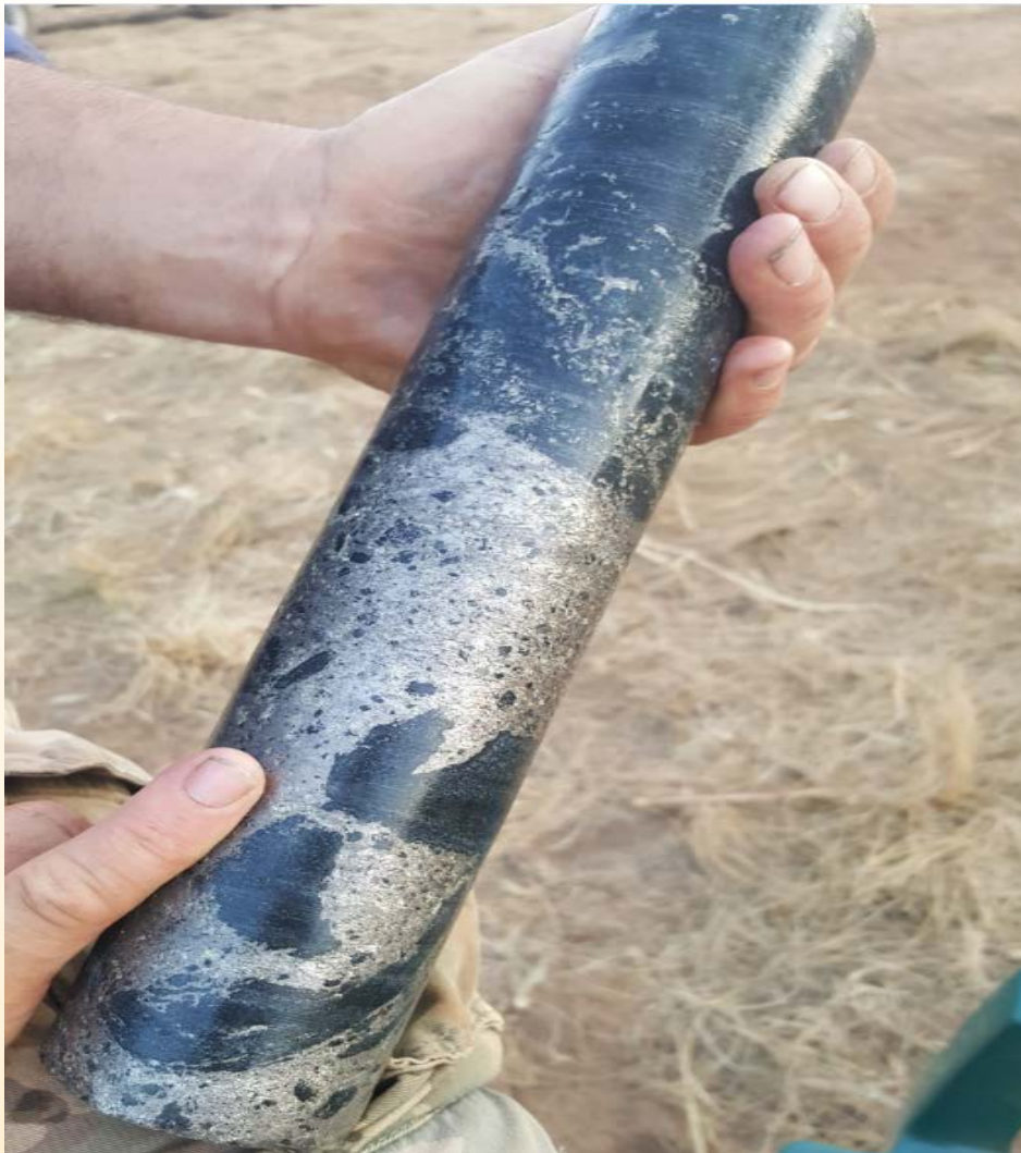
Figure 1 – Brecciated massive sulphide mineralisation in Ruins Dolerite intersected in DMDD0014, photo is of uncut HQ core, 318.5m to 319m downhole
